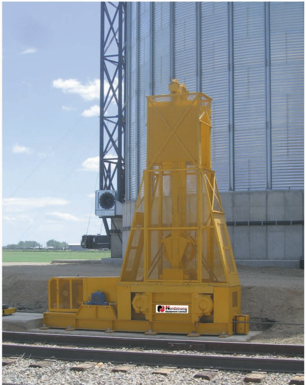
MODEL 100/125 WITH DTC DRIVE, 45,000 LBS. LINE PULL
